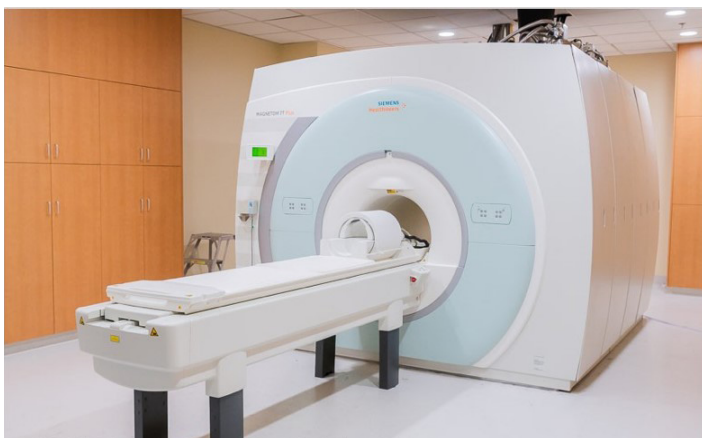
Pictured: the Siemens 7 Tesla (7T) Plus with a 60 cm bore located at the VA Advanced Imaging Research Center (VAARC). Only about 30 institutions in the U.S. have a 7T MRI and this is the only wide-bore, whole body 7T in Northern California. Photo courtesy of UCSF.
